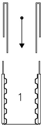
Assemble formwork units with lap joints and fix with formbraces.
